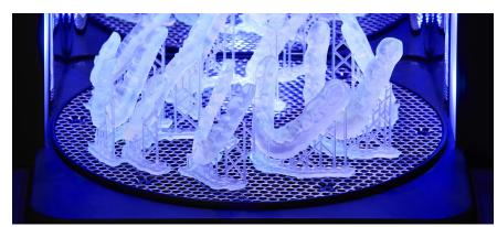
ONCE THE CHAMBER IS HEATED, 13 LEDS TRIGGER THE POST-CURING REACTION, BRINGING PARTS TO THEIR MAXIMUM MECHANICAL PROPERTIES.READY FOR OPTIMUM POST-CURING.
